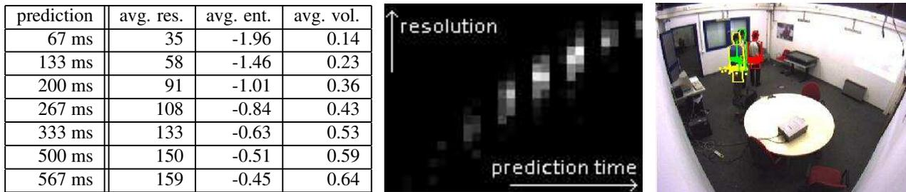
**Figure 5. Tracking with variable frame rate (sequence of 3min duration): (a) table showing average belief resolution, entropy and typical set volume for different prediction times, (b) corresponding distribution, and (c) a processed frame with propagated particles and tracker output.**
