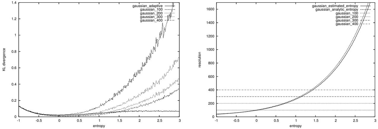
**Figure 2. Adaptive sampling on Gaussian target distributions: (a) KL divergence between reconstructed and analytic density as a function of target entropy using constant ( $n = 100, 200, 300, 400$ ) and adapted resolution; (b) number of samples drawn when using exact and estimated entropy.**
