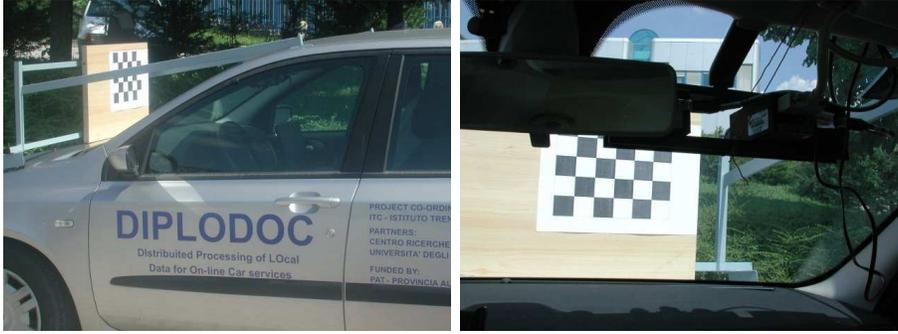
Figure 5: Extrinsic camera calibration with a checkerboard rigidly attached to the vehicle. a) lateral view (b) internal view of the three cameras looking at the calibration device.
